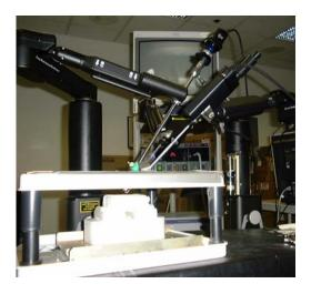
**Figure 5.** Zeus slave configuration: two instrument positioners and one endoscopic positioner inserted into an endoscopic trainer box.
