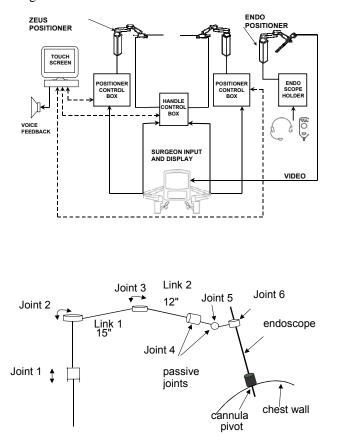
**Figure 1.** Above: block diagram showing Zeus system components. Below: Zeus positioner robot link diagram. Endoscopic robot shown; instrument robots are similar.
