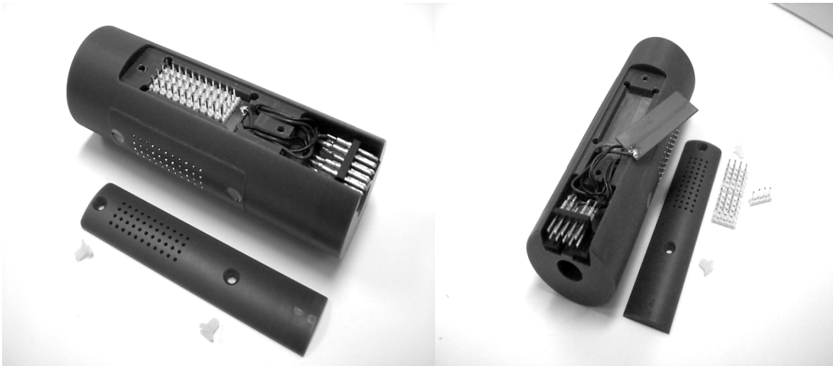
Figure 2: Disassembled Vibrotactile display revealing piezoelectric beam, cavity in which it vibrates and floating array of pins.
