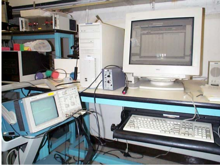
Figure 7: Data collection apparatus – scope (left), amplifier (middle), and computer (for manual recording)
