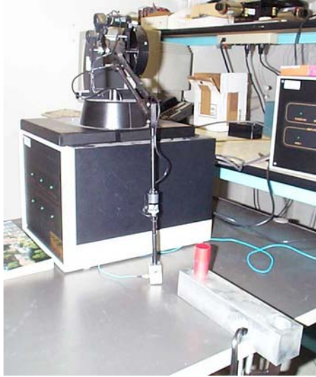
Figure 5: Experiment test-bed – PHANTOM robot atop its amplifier, sensing object attached to the stylus, and the block and peg to standardize arm and hand position
