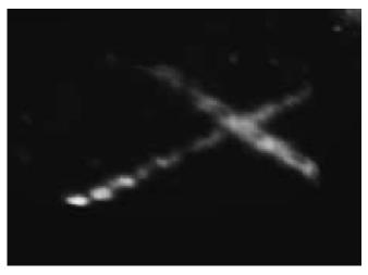
Fig. 5. 3D ultrasound image of the target X. The target was composed of two intersecting strands of nylon. This fiducial was designed to be attached to surgical targets, such as a patch.
