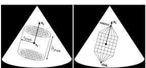
Figure 3: Example of cylindrical boundary for the graph (left) and a 2D representation of graph position and orientation along with the source and sink nodes (right).
