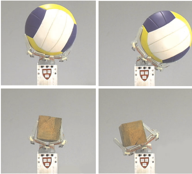
Fig. 6. Adaptability of the hand to variations in object location (i.e. centered and off-centered).
