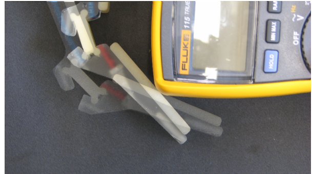
Fig. 1. Multiple exposures illustrating the use of compliant joints and joint-angle sensors to determine object geometry. Such a system is robust, inexpensive, and well-suited to the challenges of unstructured environments.
