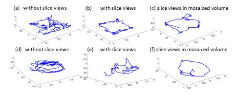
**Fig. 8.** Typical instrument tip trajectory. (a) - (c) Trajectory of tracing the rectangle rubber bands. (d) - (f) Trajectory of tracing the mitral annulus.
