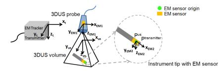
Fig. 2. Coordinate transformations for instrument tip location
