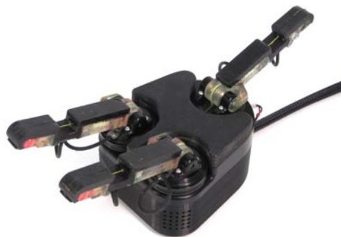
Fig. 1. The iHY Hand is an underactuated hand capable of performing a wide range of tasks, including fingertip grasping and a set of dexterous manipulation primitives.
