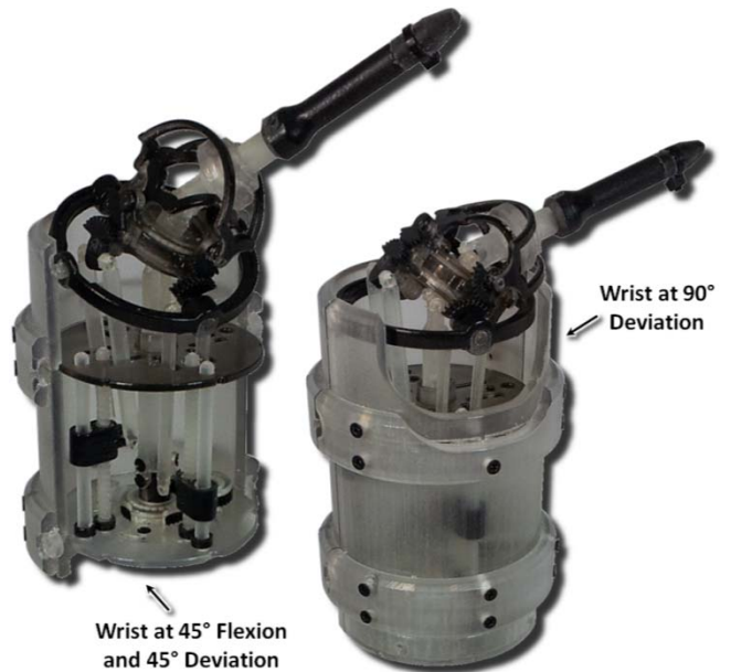
Fig. 14. Photo of the rapid-prototyped dexterous robotic wrist at 45° in both flexion and deviation (left) and at the 90° limit of lateral deviation (right).
