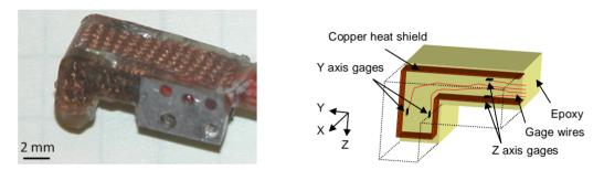
Silicon strain gages (1 mm  $\times$  0.25 mm, SS-037-022-500P, Micron Instruments, Simi Valley, CA, USA) were used to achieve high sensitivity in a small package. Individual strain gage resistances were sensed through a Wheatstone bridge, followed by an instrumentation amplifier circuit with a gain of 100.
