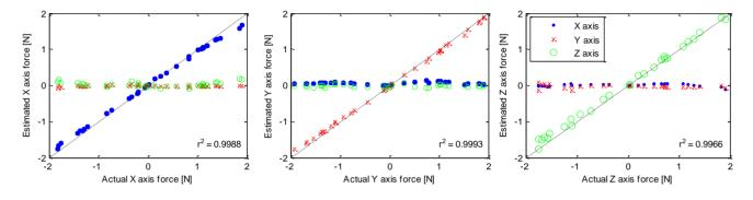
Figure 4. Sensor response to loads showing linearity.
