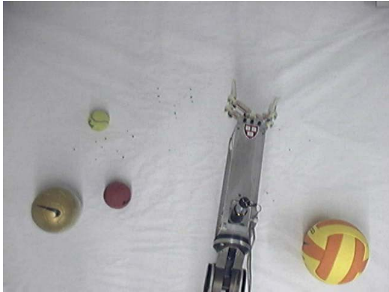
Figure 7.6. Overhead image of the workspace showing the four target objects and the robot arm. Images of the workspace taken from this camera were used to find the target object location and size.
