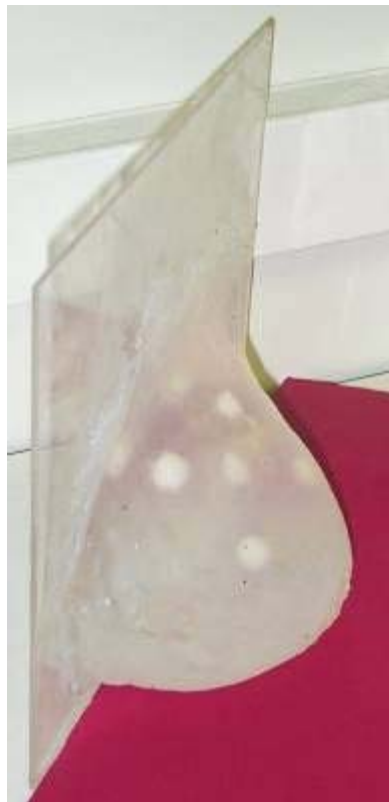
Figure 5.15. Model breast constructed to test our registration algorithm. The model is made of GE RTV 6166 two-part silicone, with modulus of elasticity if 15kPa. Rubber spheres are incorporated into the model to provide registration points. The model is coated with GE RTV 108 silicone to simulate skin and glued to a plexiglass sheet to simulate the chest wall.
