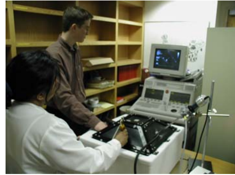
Figure 2.6 Tank study setup. In this arrangement, the surgeon (white coat) cannot see the task inside the tank except by viewing the US image on the monitor.
